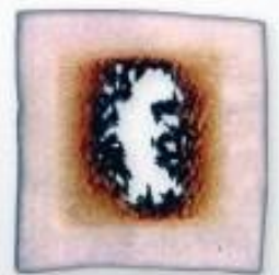
Meta aramid (100%) media after 5 sec. direct flame exposure
